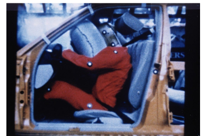
1 / The airbag increases \Delta t so as to reduce F = \Delta p / \Delta t .
